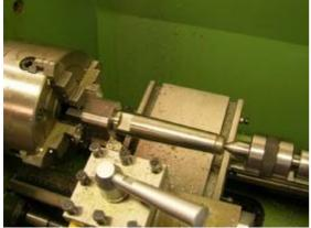
After finishing both buffer housings I swapped the chucks over and proceeded to turn the ends of the buffers from a 1.5" round bar and a <sup>3</sup>/<sub>4</sub>" round bar, which I used as the arm protruding from the buffer housing. Once the buffers were completed I assembled my "kit" of parts to produce the competed tender chassis.
