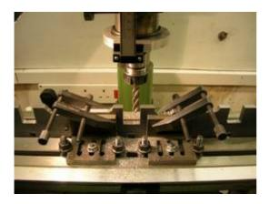
Next I machined all the frame stretchers. These all had to be milled to the same length, which I was able to do after some careful arrangement in the vice. As I was trying to build a semi-scale Q1, the outlines of the stretchers were along similar lines to those found on the real thing.
