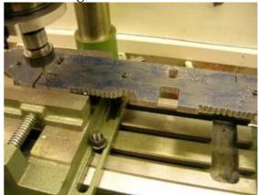
After taking some advice, I started again, but this time I clamped the bar differently, and moved the frame outline in 100thou from the edge. Next I drilled holes all around the chassis frame outline, and then used the mill to machine to the chassis frame outline. This time everything worked. So purchasing 12ft of steel was worth it !! Once the frame outline was finished, I machined out the locations for the suspension and the positions of the axles in preparation for the horn blocks.
