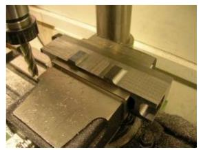
This buffer beam block was a particular challenge, as I used a fly cutter for the first time to reduce the thickness of the block down to  $1.5'' \times 1.25''$ . After this I proceeded to hollow out the block using slot and round nose mills.
