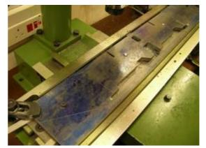
Unfortunately, my first learning experience was that by only machining one edge, both chassis frames warped and twisted, so my first effort was consigned to the scrap bin. This problem is partly due to the stresses induced during manufacture.
