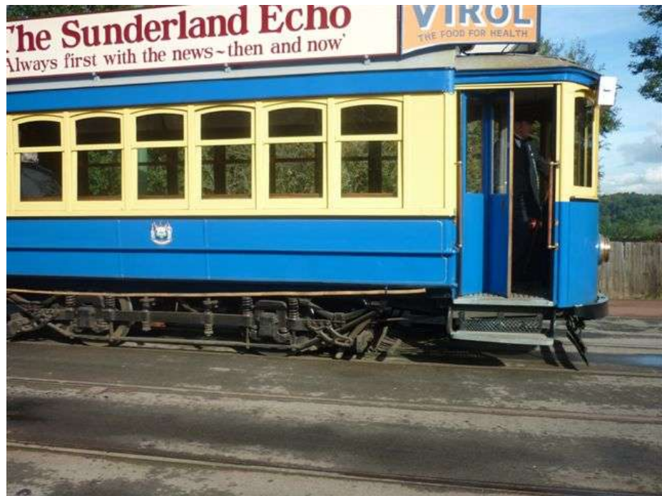
A later Tram with enclosed driver platform
