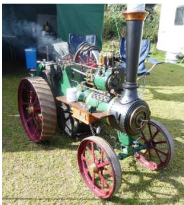
Photo 1 – 4 ½” Burrell Agricultural TE built and owned by Jon Poulter. This engine was scaled up from plans provided by Live Steam.
