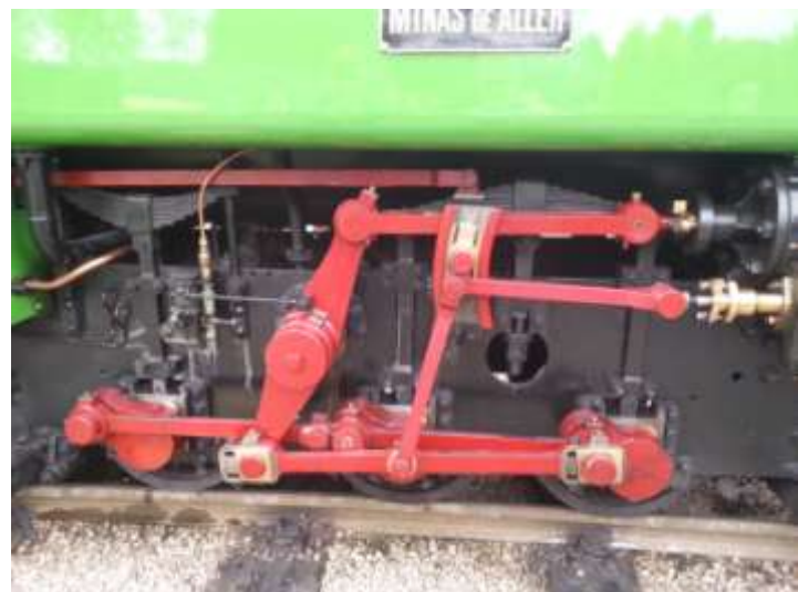
An interesting drive mechanism – Minas de Aller built by Corpet, France in 1884
