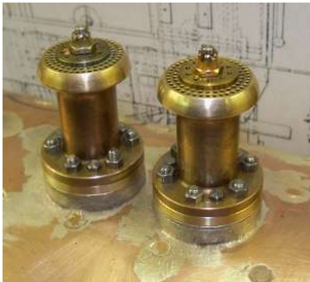
Fig 11 Model Ross POP Safety Valves 1/8 Scale
